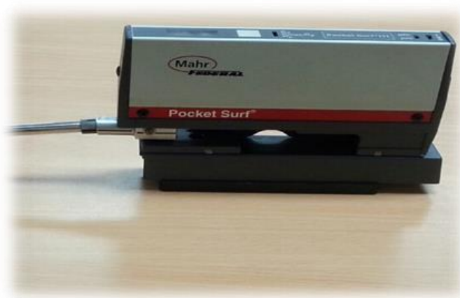
Fig. 4. Profilometer used for measuring surface roughness of ceramic
