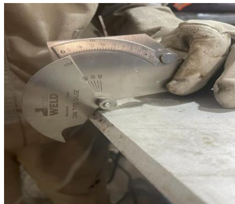
Fig. 1. Beveling of plates before welding
