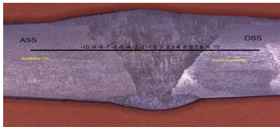
Fig. 2. Microhardness map of the cross-section weldment
