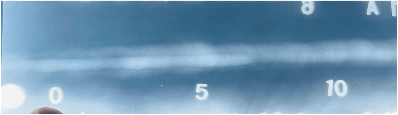
Fig. 5. Radiographic test results of the welding coupon
