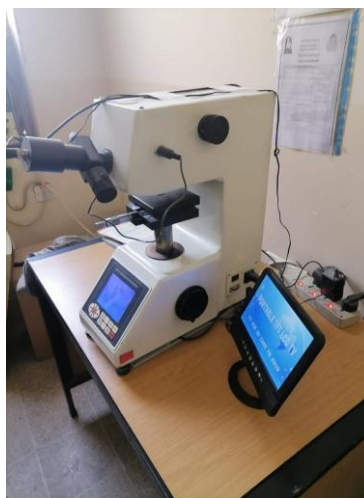
Fig. 3. Vicker microhardness device used in the test
