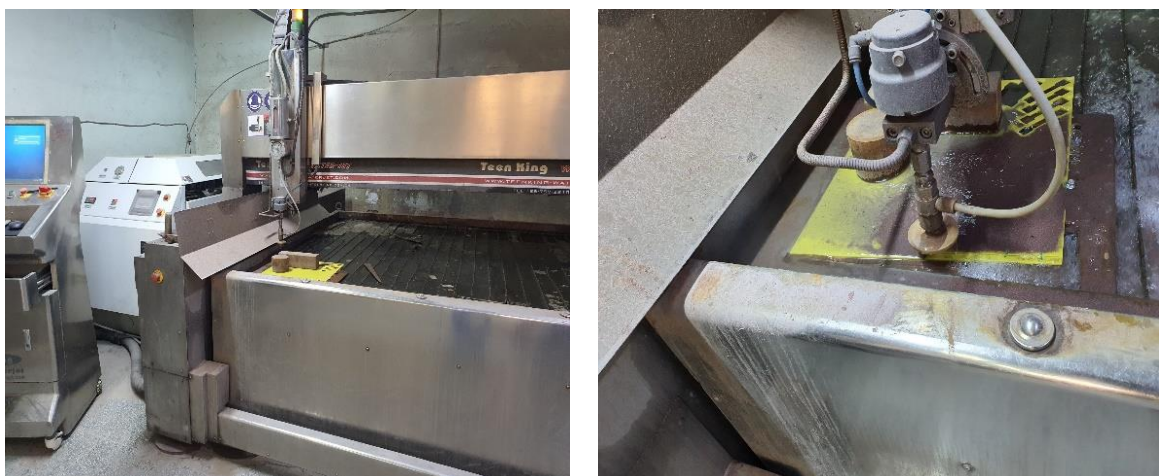
Fig. 2. CNC Water Jet Cutting Machine (flow 45o CNC Water Jet Cutting Machine)
