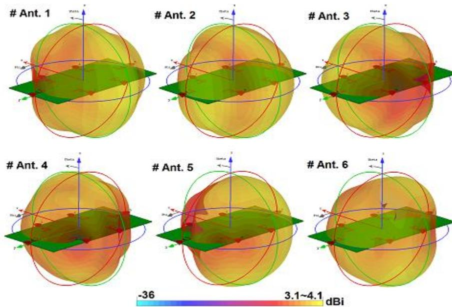
Fig. 8. The proposed MIMO antenna's 3D radiation patterns are at 3.6 GHz
