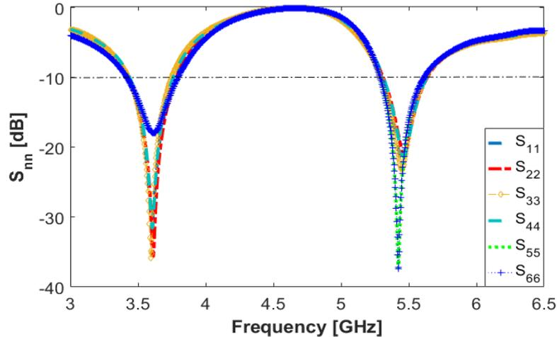
Fig. 3. Simulation of the MIMO antenna array's return loss ( $S_{nn}$ )
