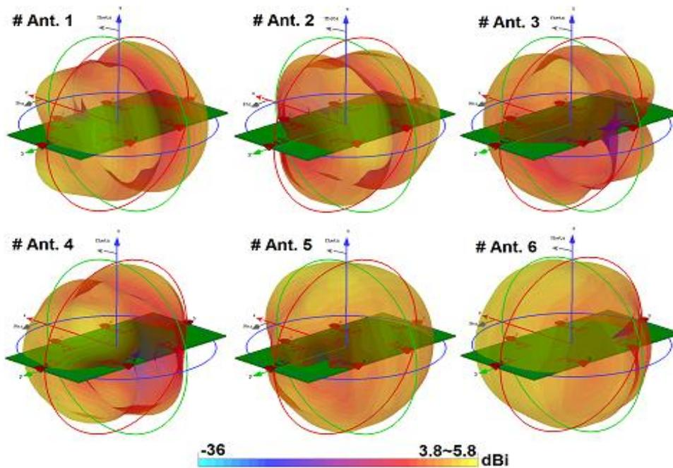
Fig. 9. The proposed MIMO antenna's 3D radiation patterns at 5.45 GHz
