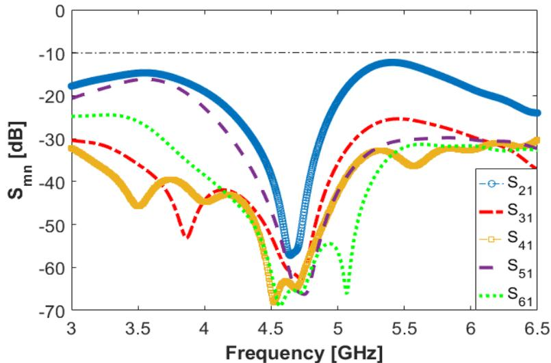
Fig. 4. Simulated result of MIMO antenna array's mutual coupling ( $S_{mn}$ )
