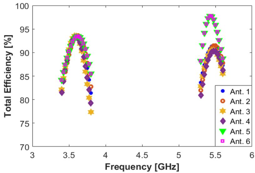
Fig 11. Overall MIMO antenna efficiency across its operating band
