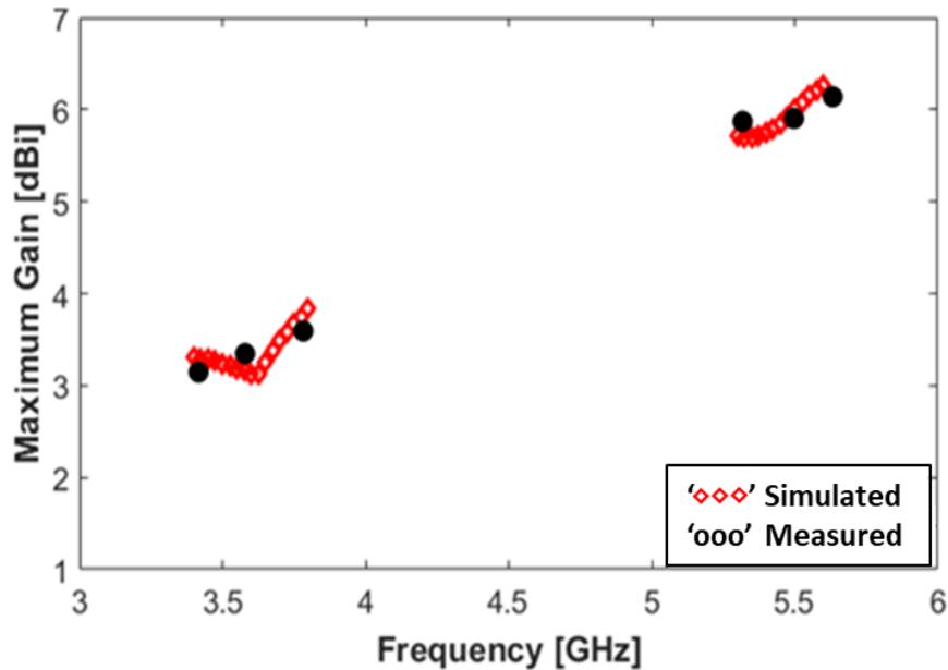
Fig. 12. Measured and simulated Maximum gains of the MIMO antenna over its operation band
