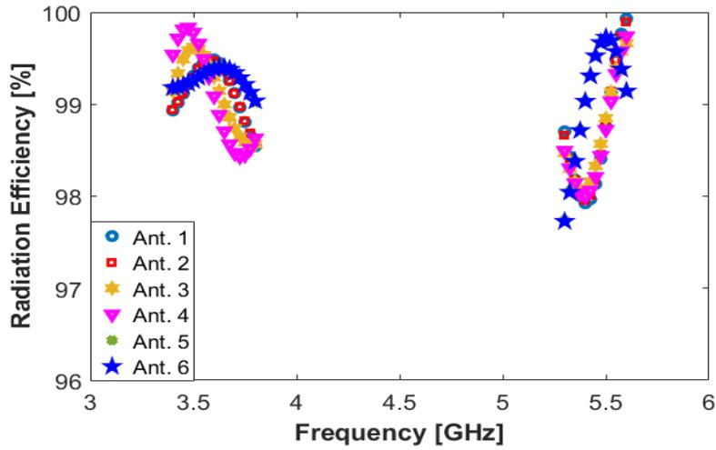
Fig. 10. MIMO antenna's radiation efficiency over its operating band
