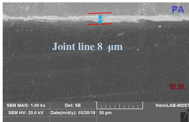
Fig. 9. SEM of the joint area for the optimum condition (50 μm)
