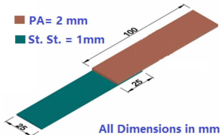
Fig. 1. Schematic lap joint of stainless steel/ polymer
