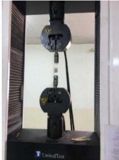
Fig. 3. Shear test equipment
