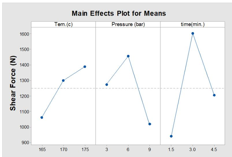
Fig. 5. Main effects plot for joining parameters
