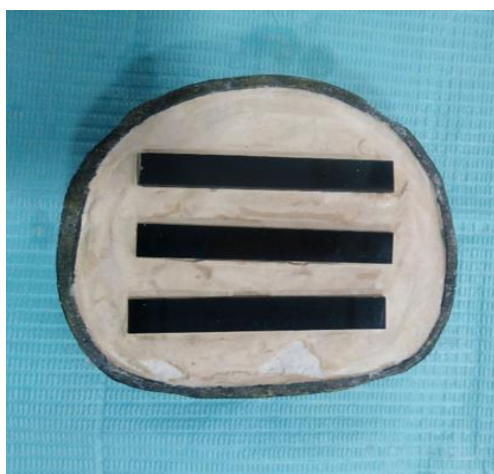
Fig. 2. Plastic patterns positioned in the lower half of the flask
