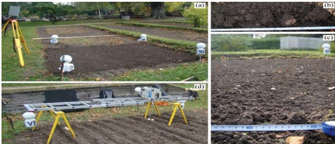
Fig. 3. (a) TLS instrument measurement setting across the investigated plot, (b, c) soil aggregates and other roughness components inside the plot, (d) optical triangulating scanner (OTS) instrument measurement configuration [ 8]
