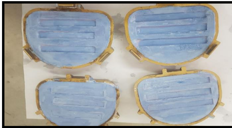
Fig. 2. Mold preparation for impact test specimens
