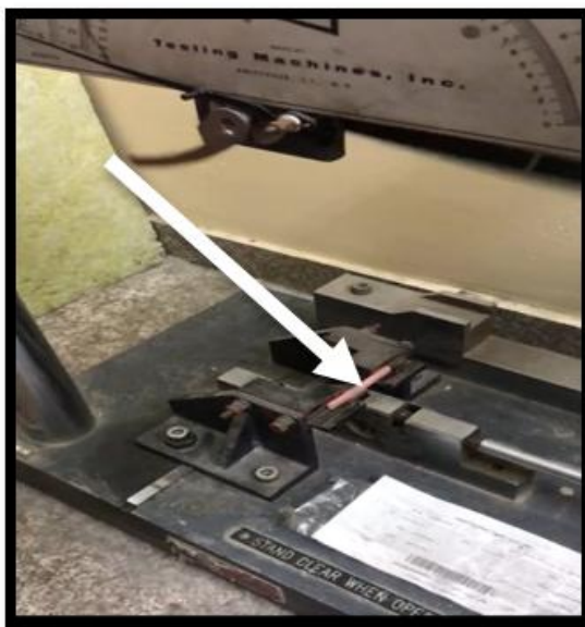
Fig. 3. Before impact testing, a position the sample in the test device (Charpy type)
