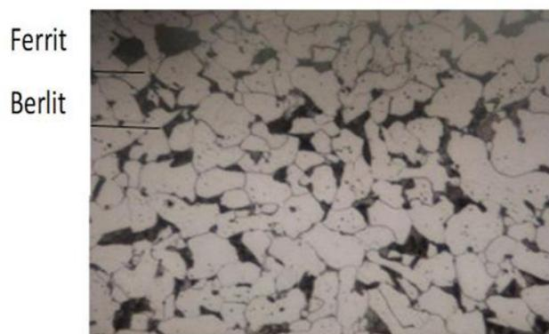
Fig. 1. Microstructure of base metal at 40X
