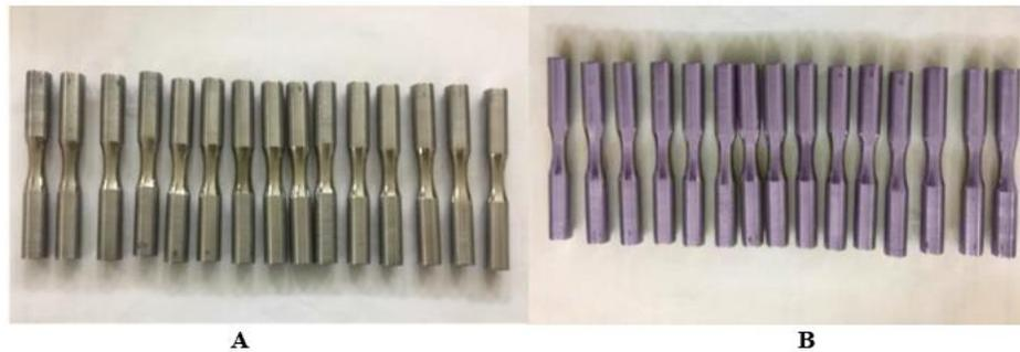
Fig. 4. Fatigue Specimens; (A) before nanocoating, (B) after nanocoating
