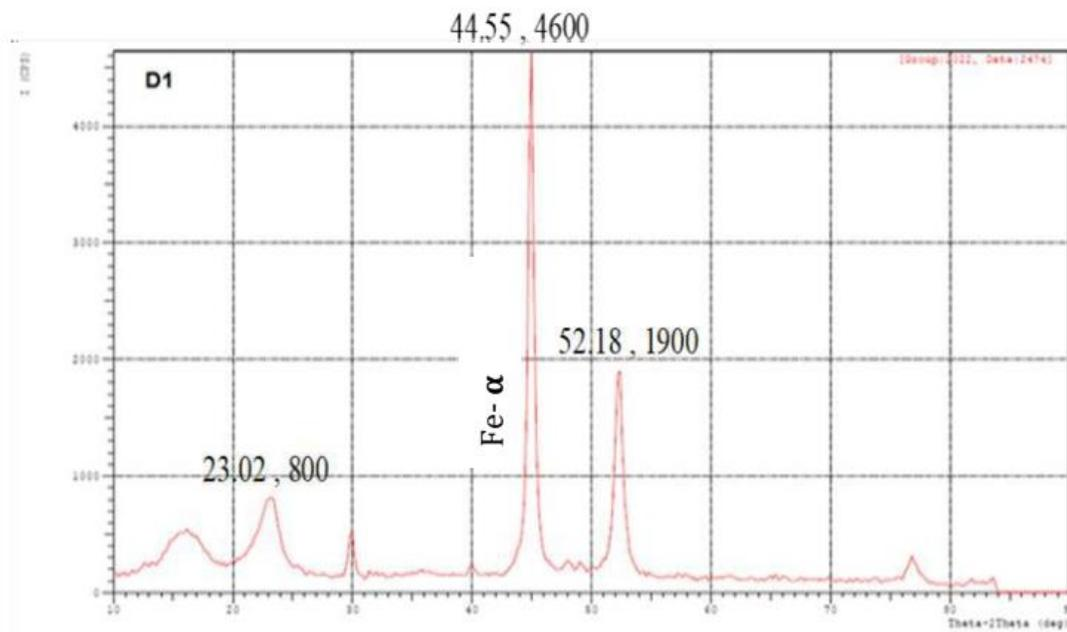
Fig. 5. XRD result of specimens (A, B1, C1, D1)
