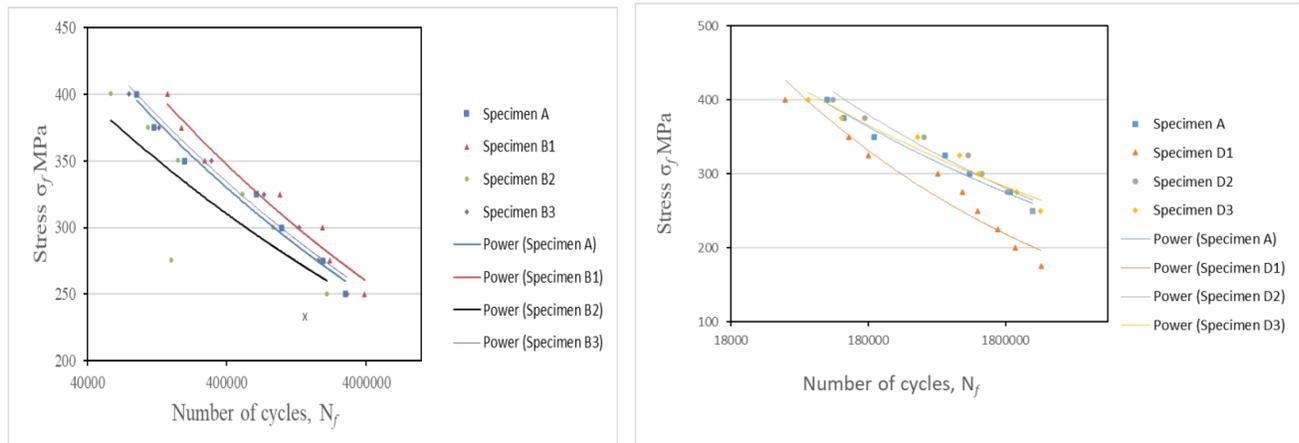
Fig. 7. S-N curves for all specimens at 0.5%nanonickel at different current density as compared with specimen(A)
