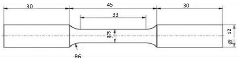
Fig. 2. Tensile test (dimensions in (mm))
