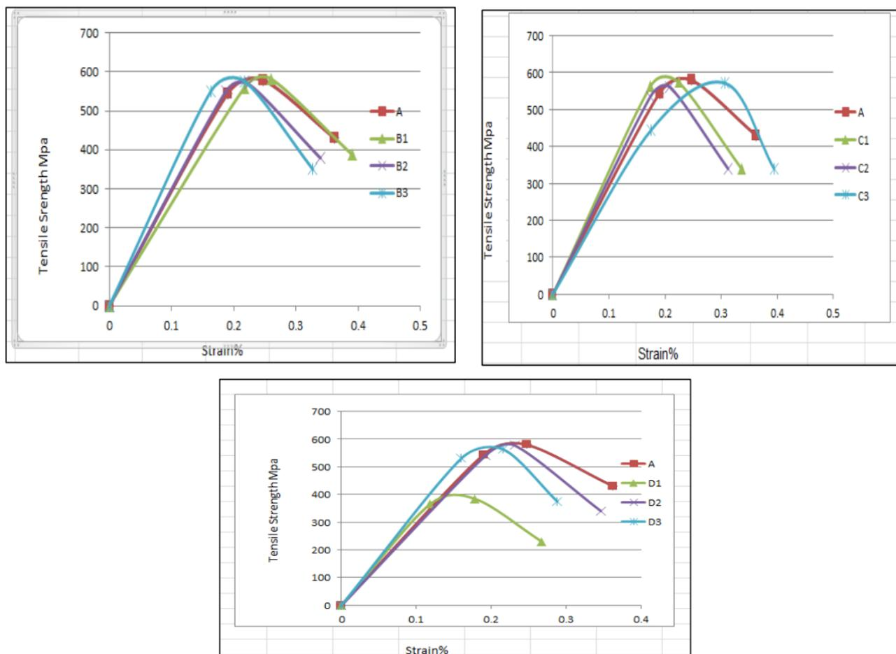
Fig. 6. Tensile test results for all specimens in Table 2
