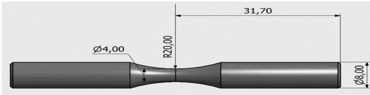
Fig. 3. Fatigue specimens (dimensions in (mm))
