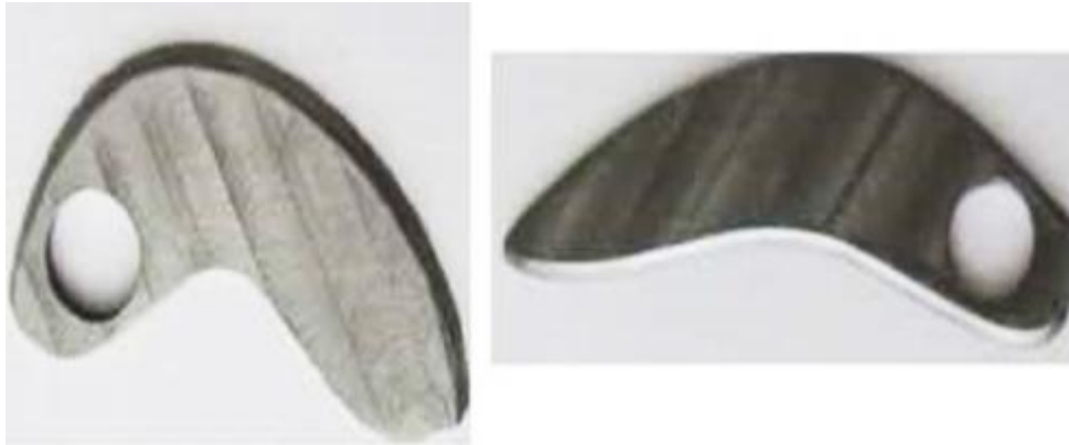
Fig. 5. Biomimetic blade (right) of Abzdak and (left) of locusts [29]
