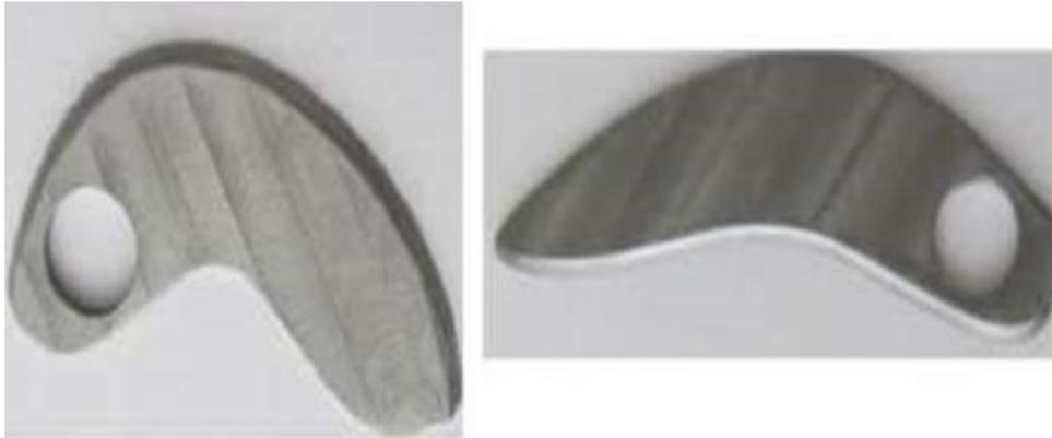
Fig. 5. Biomimetic blade (right) of Abzdak and (left) of locusts [29]
