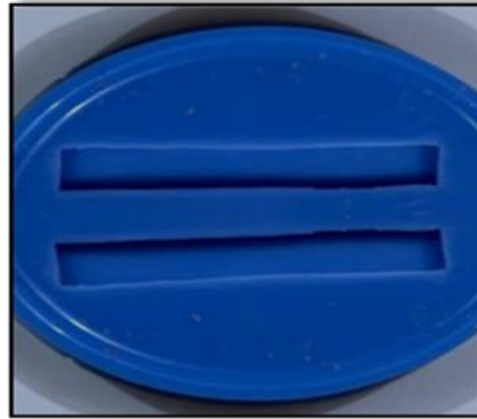
Fig. 1. Silicone mould for samples preparation
