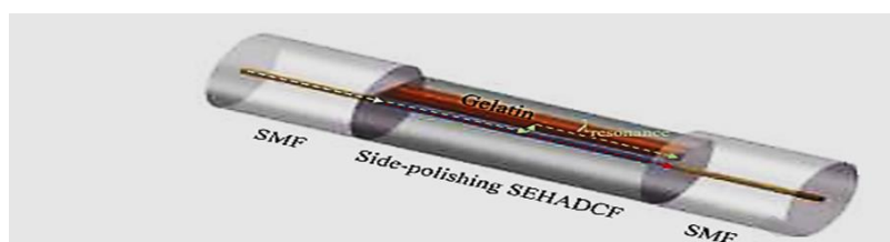
Fig. 13. RH sensor based on SEHADCF-IFDC schematic diagram, the SEHADCF's cross-section is shown inset [36]
