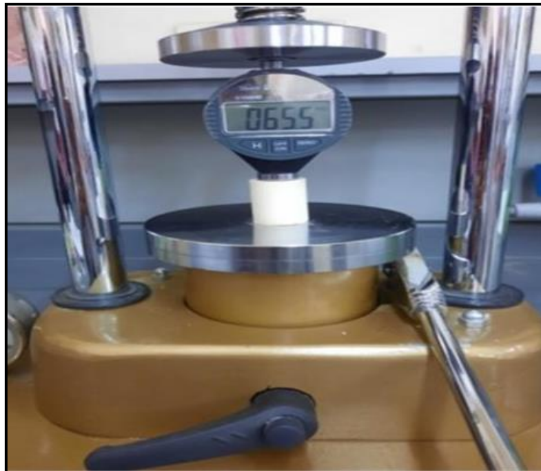
Fig. 3. The specimen's hardness test
