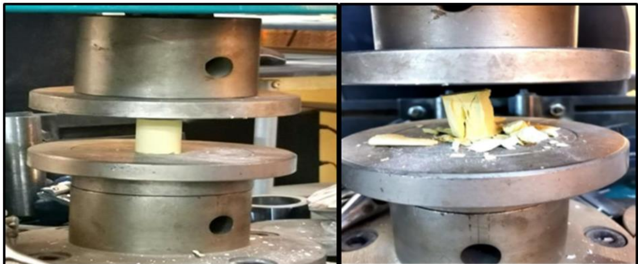
Fig. 4. Compressive strength test
