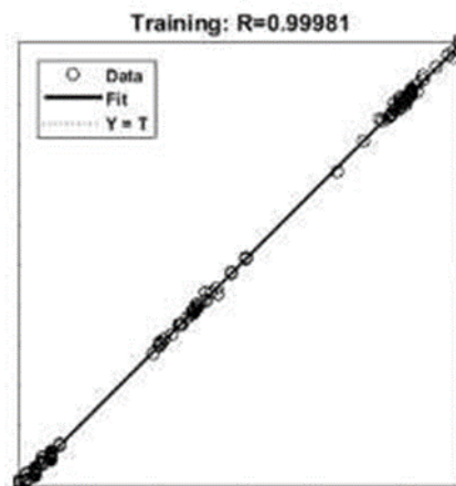
Fig. 10. Regression analysis between predicted stress and actual stress for training data
