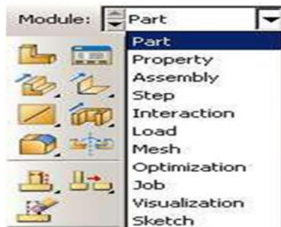
Fig. 4. Different Abaqus modules
