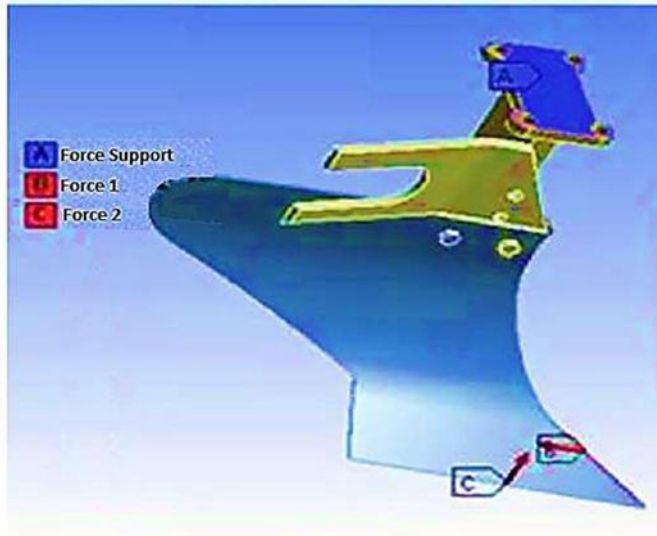
Fig. 6. Determining the place of application of force and support in the reversible plow
