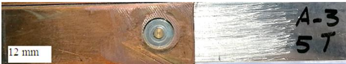
Fig. 6. The surface of the spot joint of the sample lap shear test
