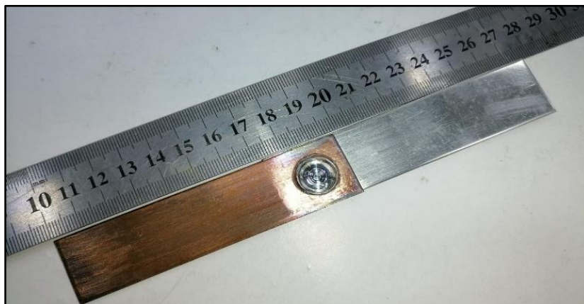
Fig. 5. The surface of the spot joint of the sample lap shear test after the welding process
