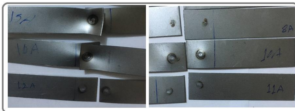
Fig. 6. After the tensile-shear test
