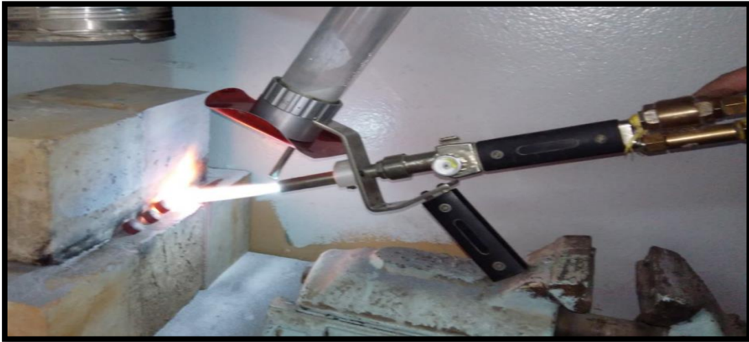
Fig. 1. The system of flam spray
