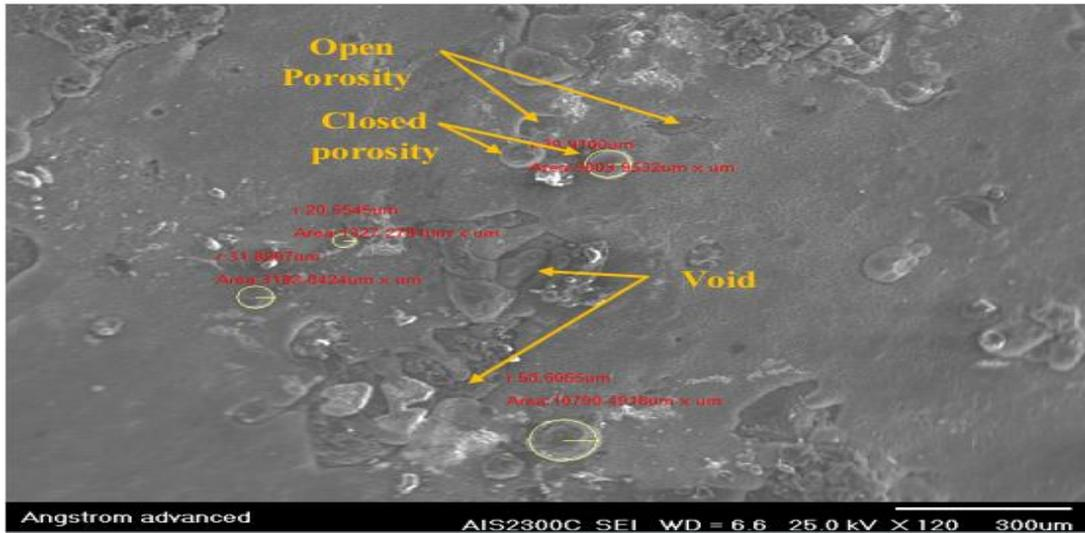
Fig. 3. SEM morphology of the flame-sprayed SiC-5wt.% Al<sub>2</sub>O<sub>3</sub> coating layer
