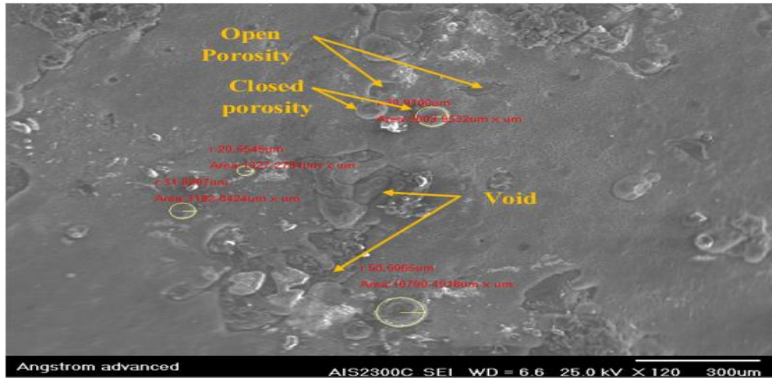
Fig. 3. SEM morphology of the flame-sprayed SiC-5wt.% Al 2 O 3 coating layer
