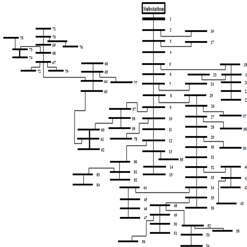
Fig. 2. The single-line diagrams for Case 2
