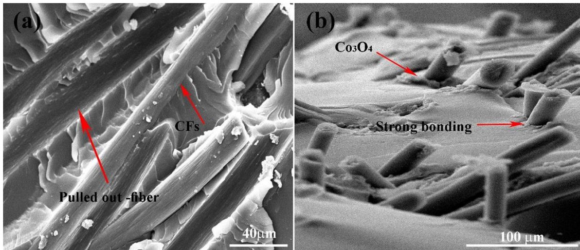
Fig. 5. Displays the fracture surface of the 3D CFs/epoxy composites, with and without \text{Co}_3\text{O}_4 nanowire; (a) Three-dimensional carbon fiber/epoxy composites, (b) Carbon nanowires incorporated into carbon fiber/epoxy composites
