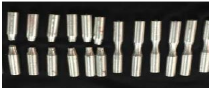
Fig. 4: Fatigue Specimens before & after Fatigue testing
