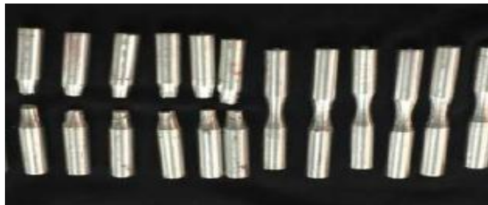
Fig. 4: Fatigue Specimens before & after Fatigue testing
