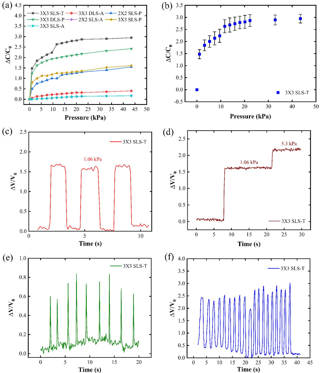
Fig. 4. (a) Relative capacitance responses of the sensors with different configurations, (b) Relative capacitance curve of three independently structured 3X3 SLS-T sensors, (c) Repeatability of the 3x3 SLS-T sensor under the same load (1.06 kPa), (d) Voltage change rate responses of the 3x3 SLS-T sensor under different pressure loadings (1.06 and 5.3 kPa), (e) Quick tapping responses of the 3x3 SLS-T pressure sensor, (f) Palm bending responses of the 3x3 SLS-T pressure sensor
