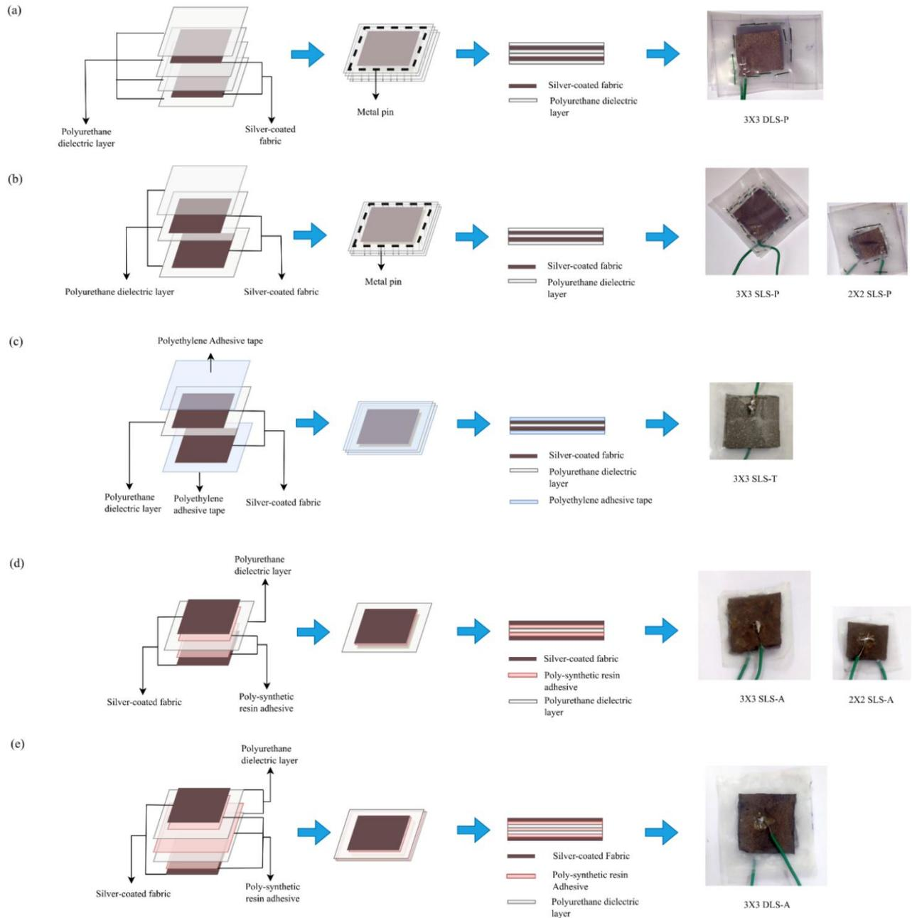
Fig. 1. The fabrication method of the flexible capacitive pressure sensors: (a) 3×3 DLS-P, (b) 3×3 SLS-P and 2×2 SLS-P, (c) 3×3 SLS-T, (d) 3×3 SLS-A and 2×2 SLS-A, (e) 3×3 DLS-A
