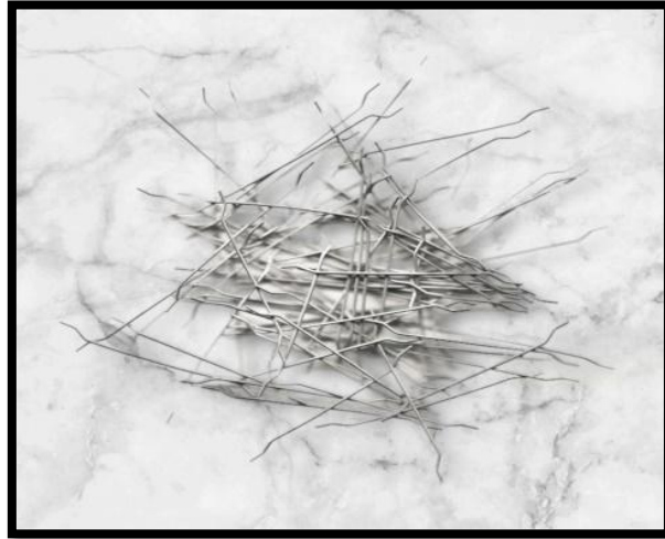
Fig. 5. The shape of the steel fibers
