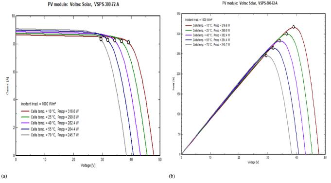
Fig. 7. The Temperature effect on the used PV panels (Model: VSPS-300-72-A), a) Current vs. Voltage@ different temperatures, b) Power vs. Voltage@ different temperatures
