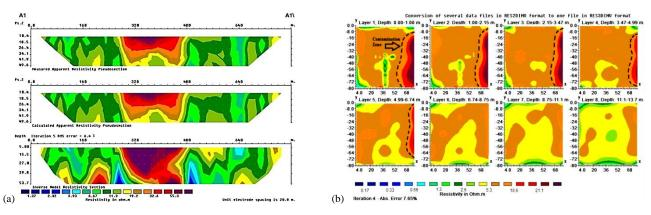
Fig. 2. Electrical resistivity imaging survey for detecting groundwater aquifer, a) Sample 2D survey image[33], b) Sample 3D survey image[34].
