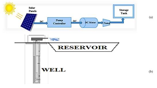
Fig. 3. Pumping unit station; a) the pumping unit block diagram, b) reservoir level.
