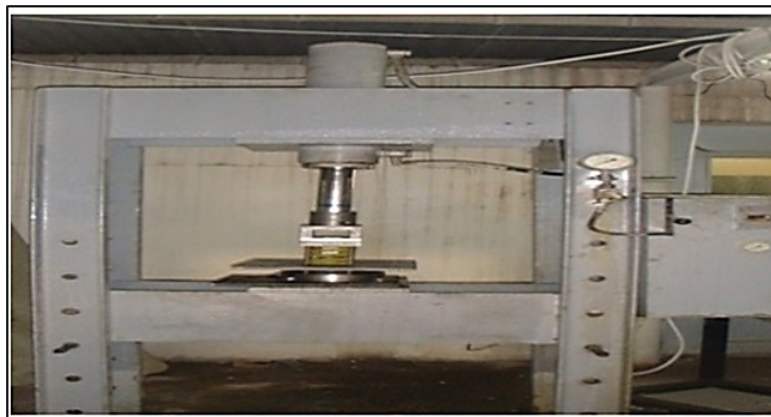
Fig. 2. The machine tool used for deep drawing experiments
