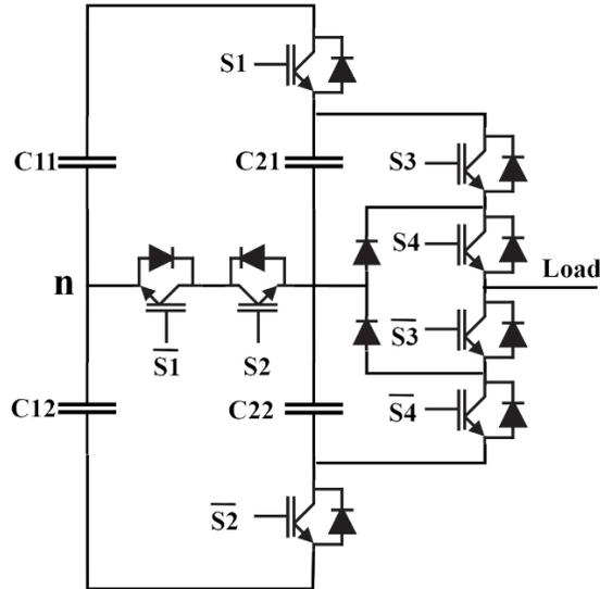
Fig. 1 One leg of ASMLI
