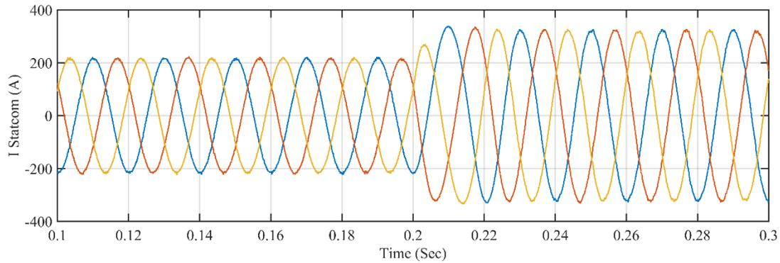
Fig. 13 The step-change in STATCOM current on a healthy network
