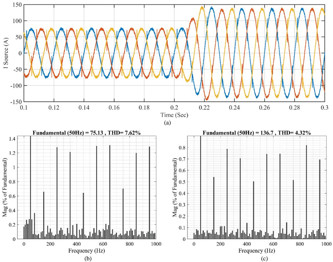
Fig. 9 System configuration with the proposed STATCOM (a) Source current, (b) FFT analysis for source current (0.1-0.2 Sec), (c) FFT analysis for source current (0.2-0.3 Sec)
