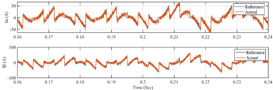
Fig. 12 Current reference tracking in stationary reference frame for two-level converter
