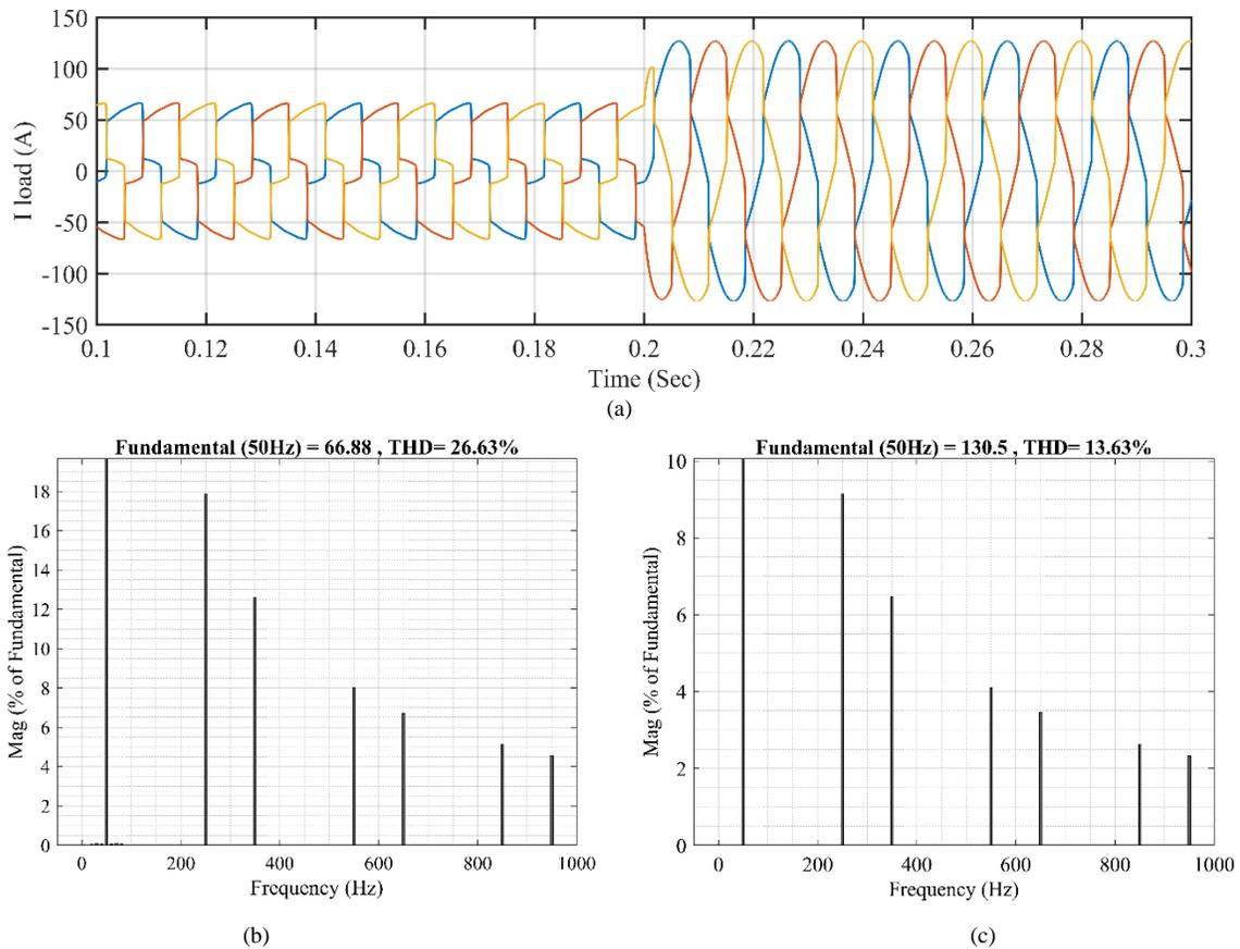
Fig. 8 (a) Load current, (b) FFT analysis for load current (0.1-0.2 Sec), (c) FFT analysis for load current (0.2-0.3 Sec)
