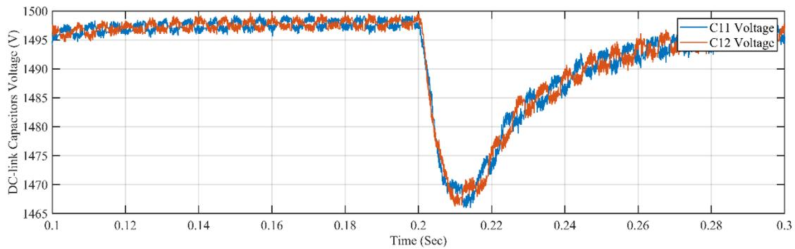
Fig. 14 DC-link capacitors voltages during a step change in load
