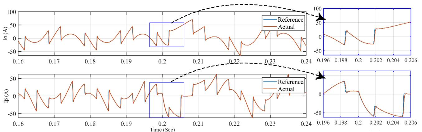
Fig. 10 Current reference tracking in the stationary reference frame for the proposed prototype
