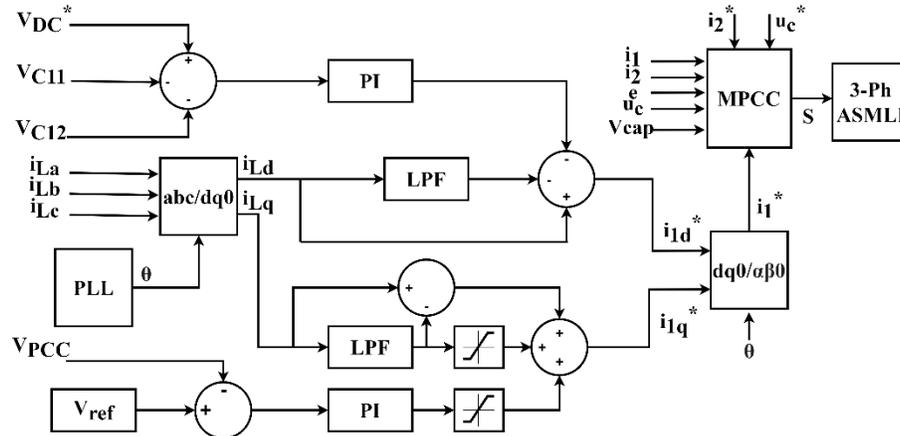
Fig. 4 STATCOM control block diagram
