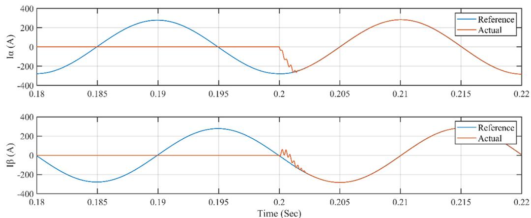
Fig. 16 Current reference tracking the moment of adding STATCOM to the network
