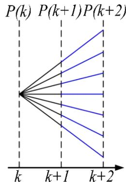
Fig. 5 Two-step prediction MPC
