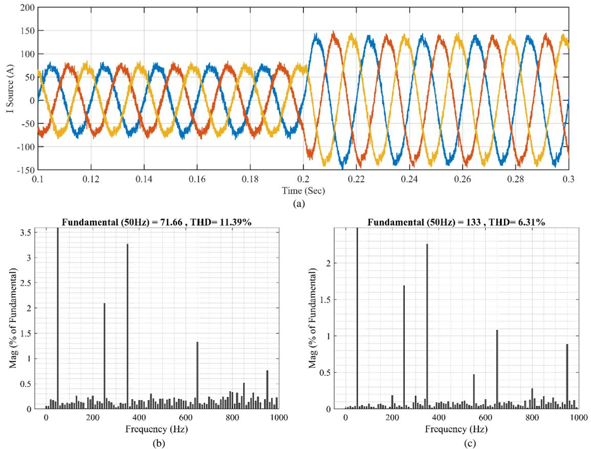
Fig. 11 System configuration with two-level converter STATCOM (a) Source current, (b) FFT analysis for source current (0.1-0.2 Sec), (c) FFT analysis for source current (0.2-0.3 Sec)
