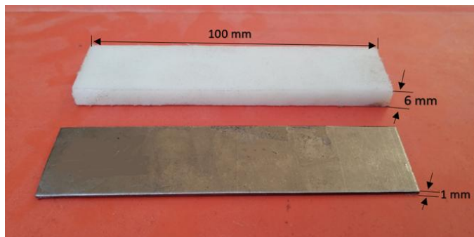
Fig. 2 Titanium and nylon 6 specimens' dimensions
