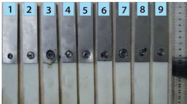
Fig. 5 Top view of specimens joining of pre-threaded Ti-g2 to nylon 6
