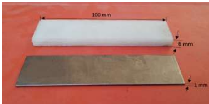
Fig. 2 Titanium and nylon 6 specimens' dimensions
