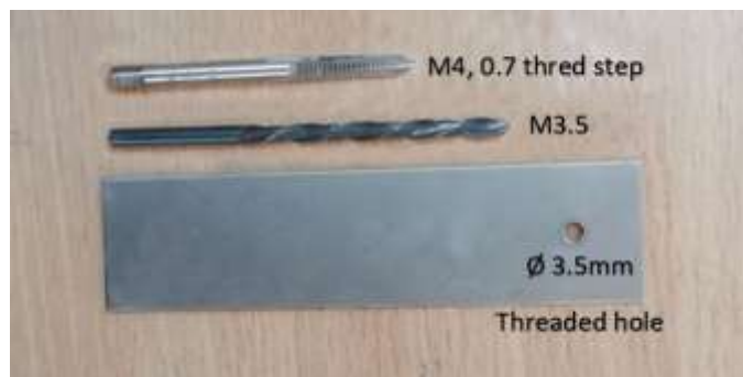
Fig. 1 Threaded hole details of titanium
