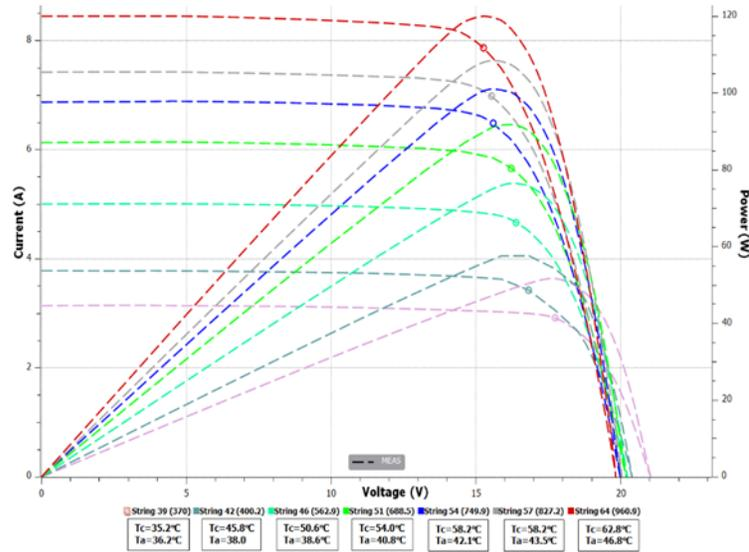
Fig 10. Measured I-V and P-V curves for the reference PV module
