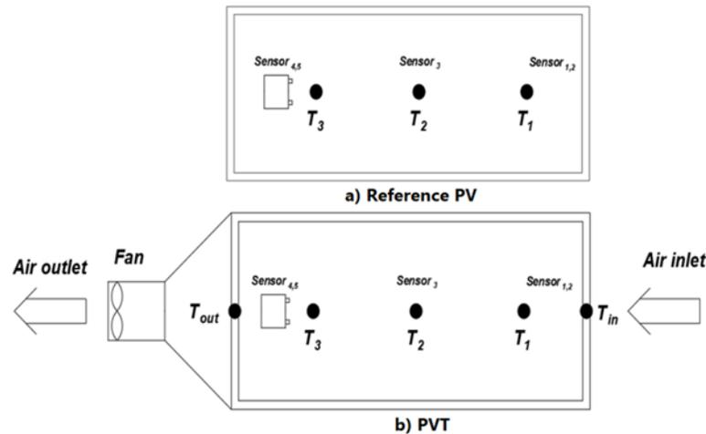
Fig 2. Sketch diagram of distributing the thermocouples
