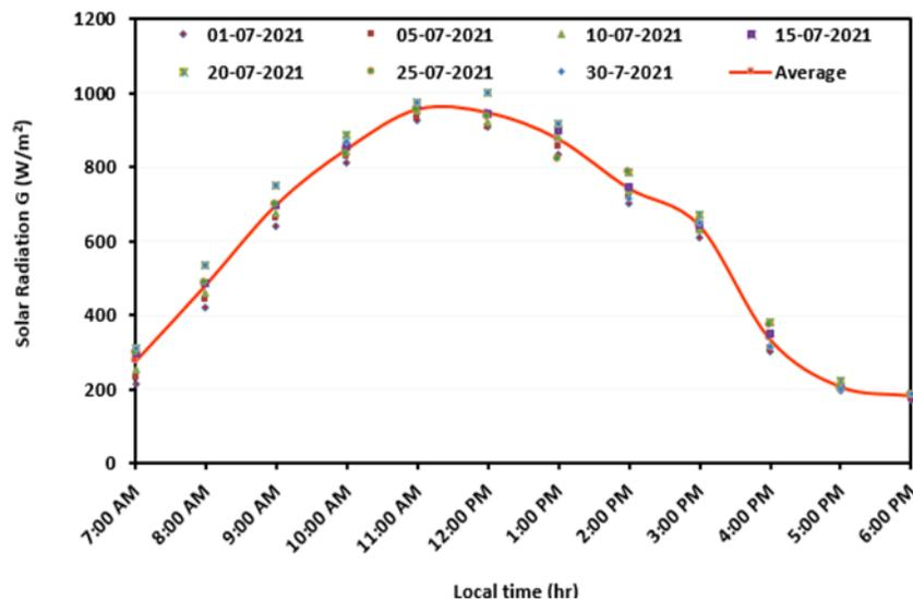
Fig 3. Variation of solar radiation with local time during July
