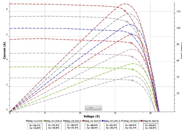
Fig 12. Measured I-V and P-V curves for the PVT module at an airflow rate of 0.155 kg/s
