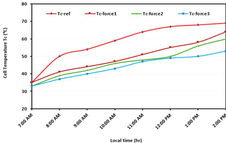
Fig 5. Variation of the back temperature of the PV module during the test period
