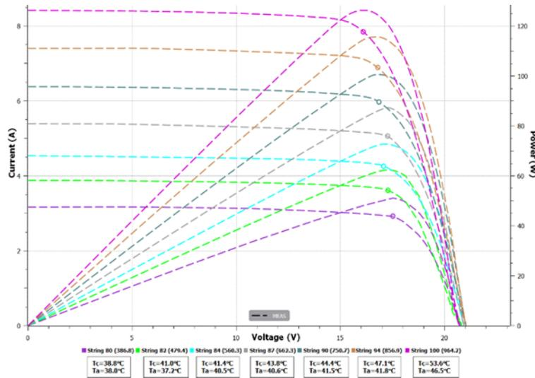
Fig 11. Measured I-V and P-V curves for the PVT module at an airflow rate of 0.093 kg/s
