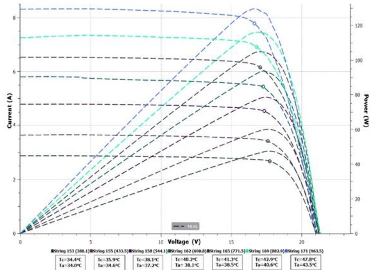
Fig 13. Measured I-V and P-V curves for the PVT module at an airflow rate of 0.22 kg/s
