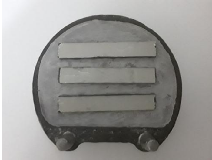
Fig 1. Plastic patterns positioned onto the stone mold
