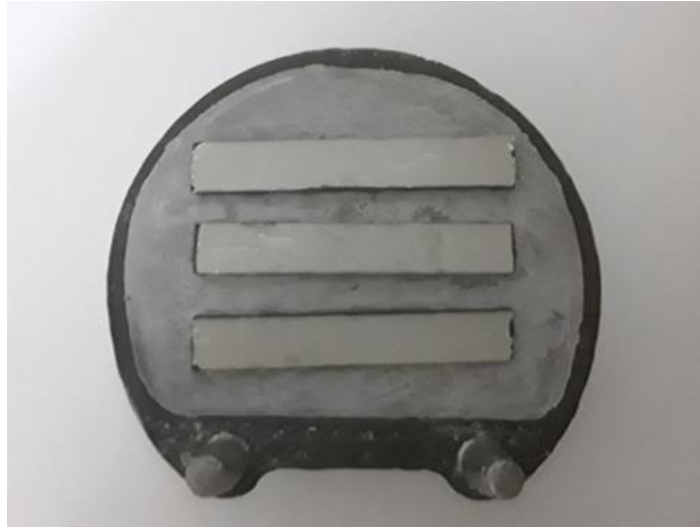
Fig 1. Plastic patterns positioned onto the stone mold
