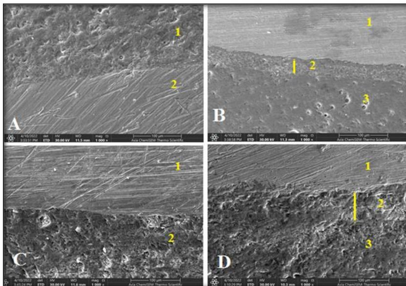
Fig 4. SEM images for metal-ceramic interface (A): casting without bonding an agent (1 ceramic layer, 2 metal surfaces), (B): casting with an agent (1 metal surface, 2 bonding agents, 3 ceramic layers), (C): SLM without an agent (1 metal, 2 ceramic), and (D) SLM with an agent (1 metal, 2 agents, 3 ceramic).
