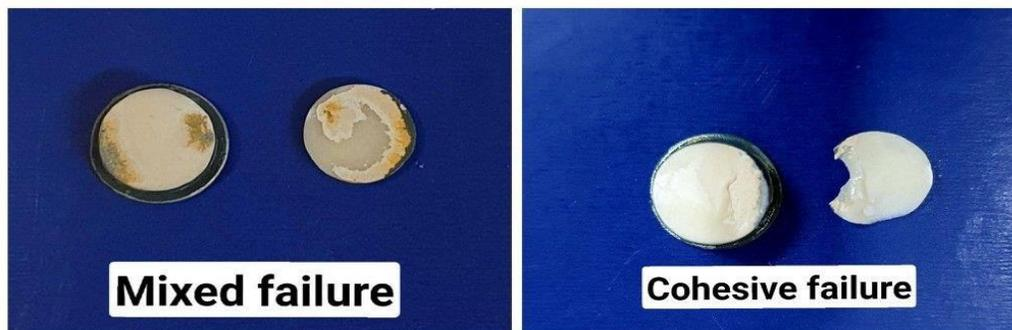
Fig 6 Shows the Co-Cr surfaces of specimens after de-bonding from the ceramic after the shear bond strength test
