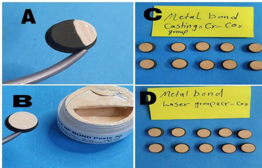
Fig 2. A and B (Vita NP Bond paste was applied to the surface of the alloy), C and D (Vita NP Bond was firing)
