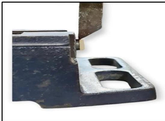
Fig 3. Chisel part of Instron universal testing machine loading the PFM interface until fracture
