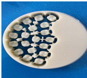
Fig 1. Interim crowns samples made from PMMA CAD/CAM disk resin after milling process
