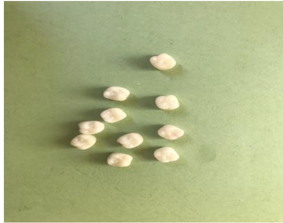
Fig 2. Interim crowns sample made from 3D printing resin after printing process
