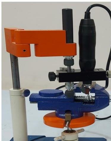
Fig 2. A specimen mounted on a dental surveyor of the finishing process in the standard method
