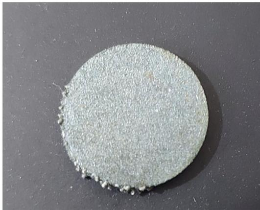
Fig 1. A printed specimen of Co-Cr made by selective laser melting (SLM) according to the adopted (. STL) file design
