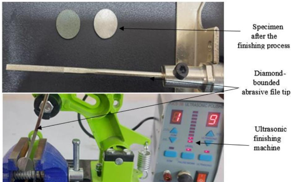
Fig 3. Finishing procedures through the ultrasonic method
