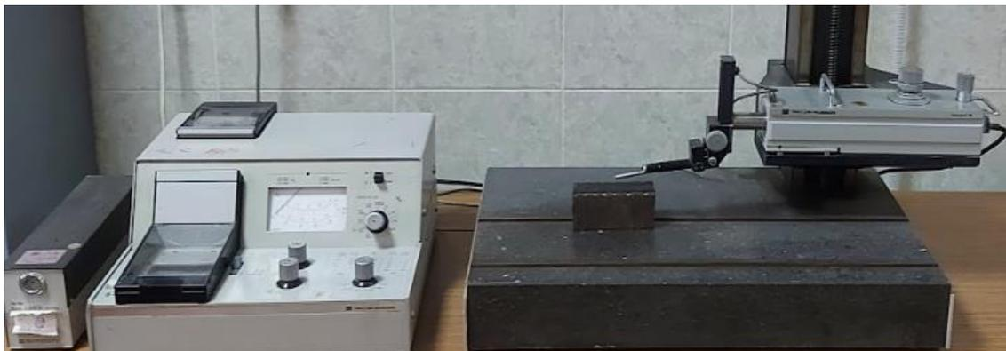
Fig 4. A profilometer (Taylor) for surface roughness testing
