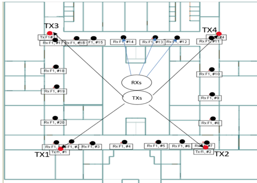
Fig. 4. The deployment of 4TXS & 20RXs
