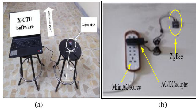
Fig. 2. The hardware of the proposed system in the indoor environment: (a) BANs and (b) MAN. BAN= Beacon Anchor Nodes, MAN= Anchor Nodes Mobile, AC=Alternating current, DC=Direct current
