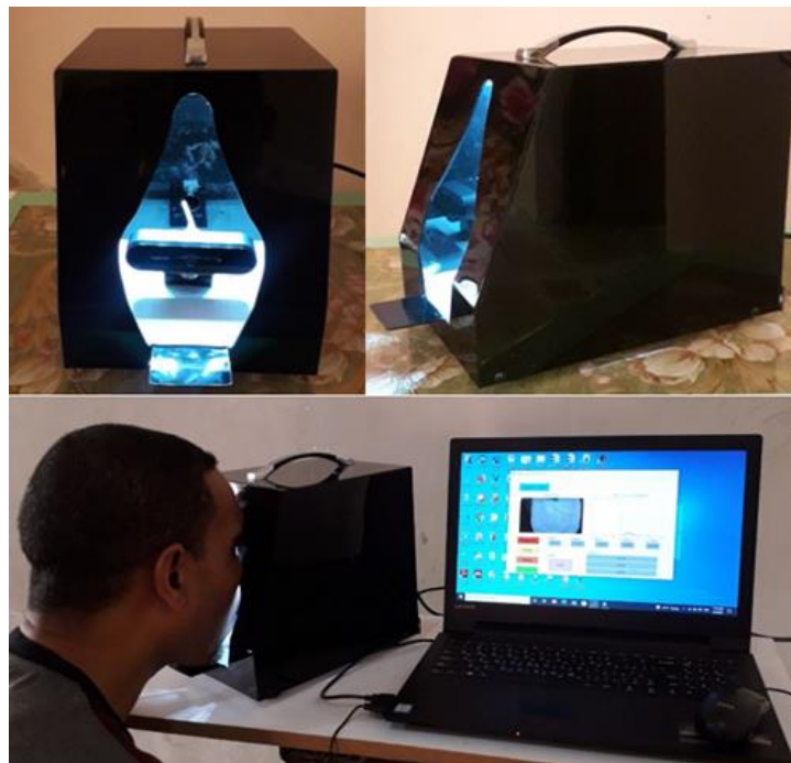
Fig. 1. Tongue image capture device and experimental setup of the proposed imaging system
