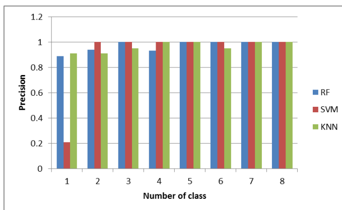
Fig. 6. Comparison of the detection precision between the proposed RF, SVM, and KNN approaches
