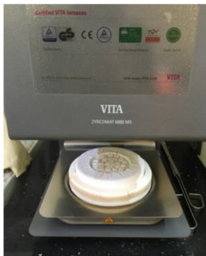
Fig. 6. Sintering furnace of Zirconia
