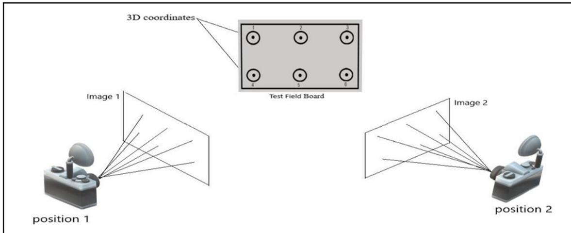
Fig. 2. Photogrammetric Test Field Board and camera capture positions
