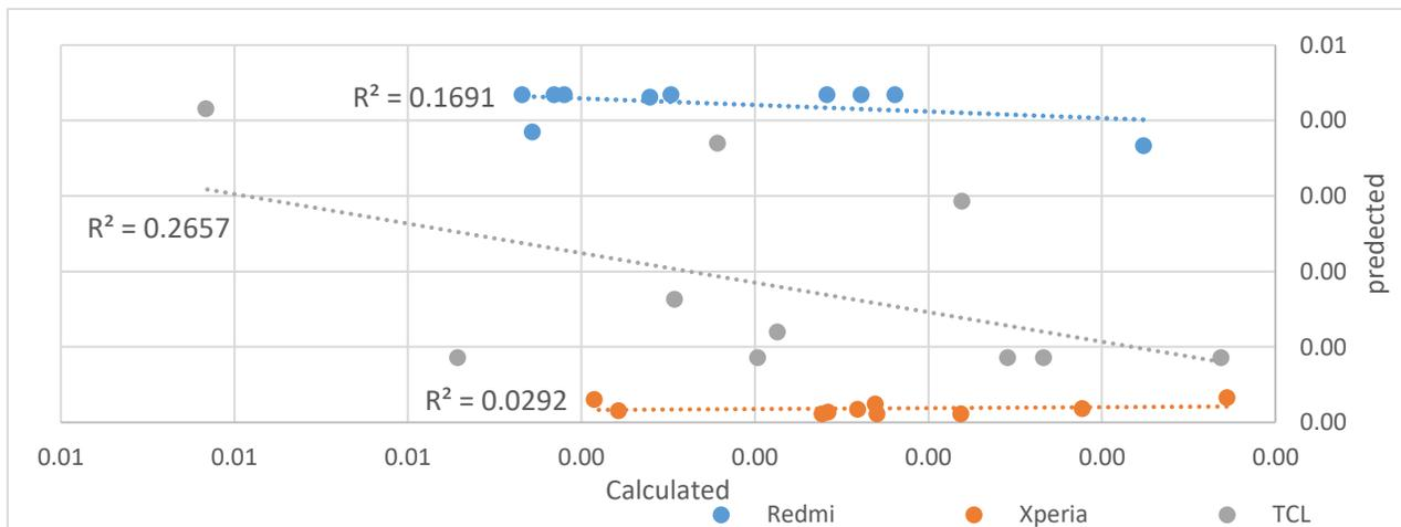
Fig. 10. The correlation between calculated  $p_1$  by self-calibration and estimated by Heuristics simulated annealing
