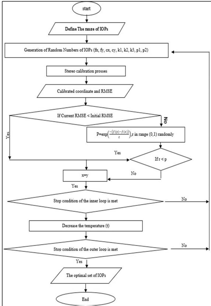
Fig. 4. Flowchart estimating IOPs by simulated annealing based on stereo calibration
